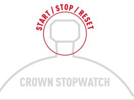
Simple time measurement with no interrupt option, i.e. start, stop and zero-setting via crown.
