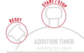
For time measurement with interrupt option, i.e. start and stop by crown, zero-setting via side button; Flyback (Tempo) over the left button optional on all models.
